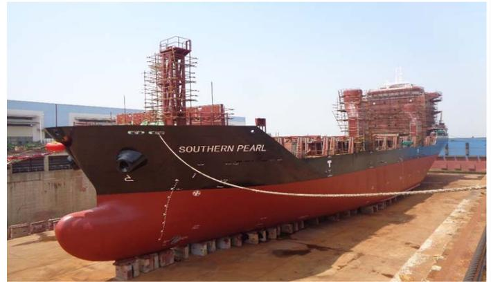
PDL's newest vessel, the Southern Pearl is nearing completion and on target for delivery in August. The purpose built ship with her shallow draft and broad beam is designed to maximise loads into the Ports of Wallis, Futuna, Funafuti, Tarawa, Suva and Lautoka. More details will be in our next Take 5 after the official launch
